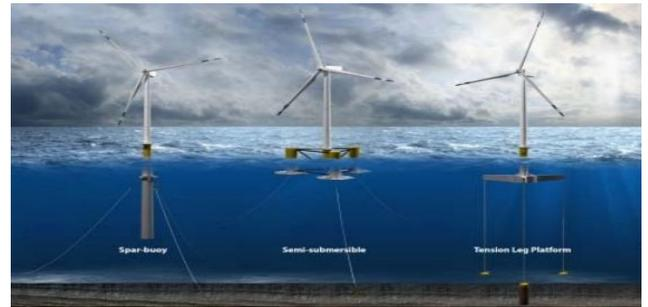
Figure 26 Different types of floating foundations.
