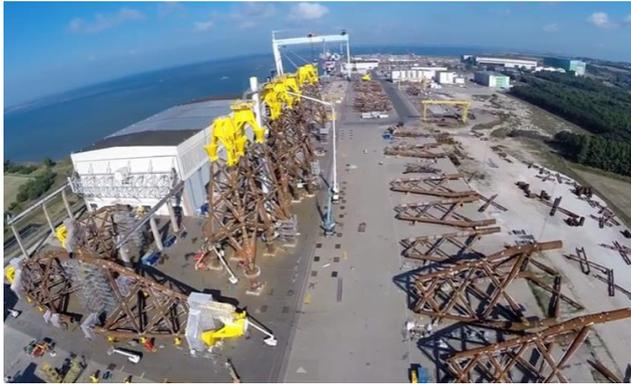
**Figure 10** Bladt Industries jacket manufacturing, Denmark.
